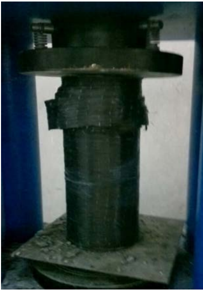
Plate 1: Two layers CFRP wrapped columns
